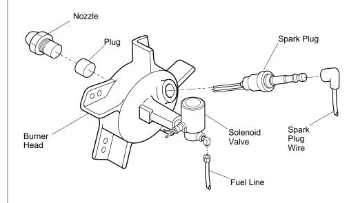
Figure 9 - Replacing Nozzle
